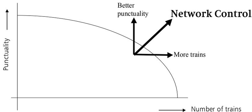
Figure 2: Objectives of Network Control
