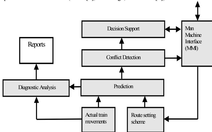
Figure 1: CD/DS System architecture with off-line diagnostic analysis
