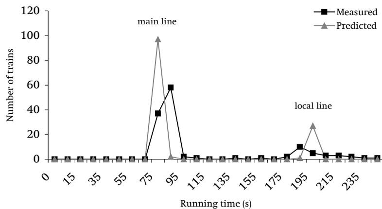
Figure 4: Measured and predicted running times between two signals
