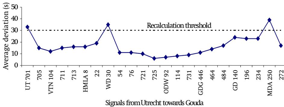
Figure 3: Average deviation between measured and predicted signal passing times
