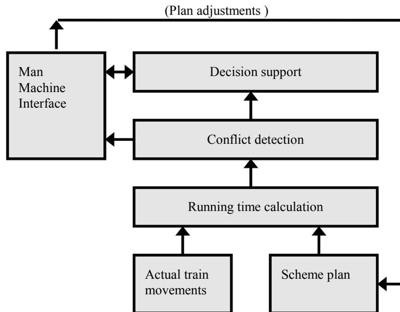
Figure 1. System architecture CD/DS system
