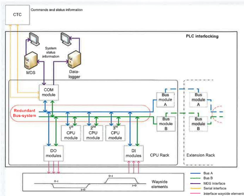
Figure 3: System architecture
